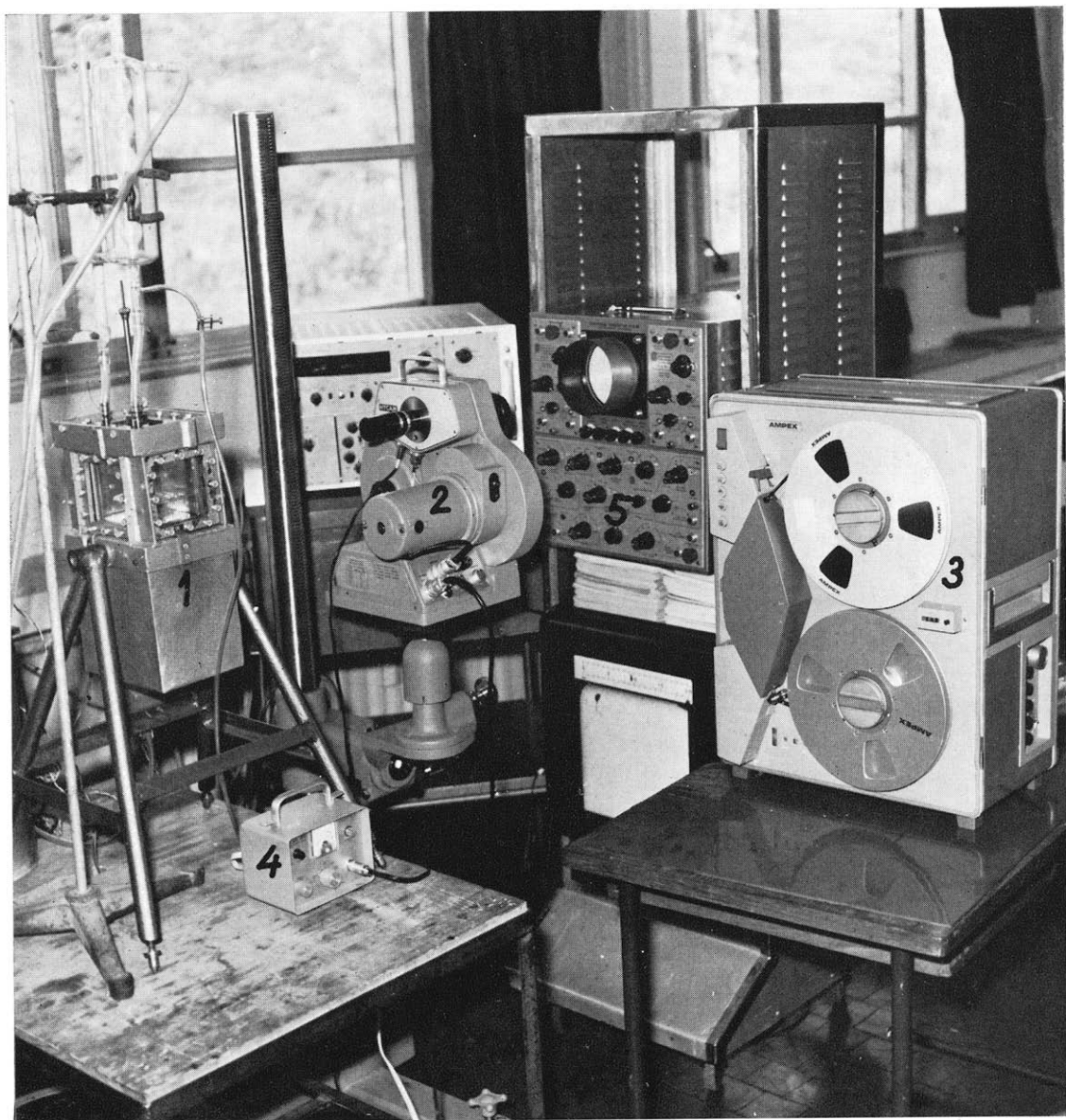
FIG. 1. Experimental set-up of boiling vessel, high speed camera, magnetic recorder and oscilloscope.
